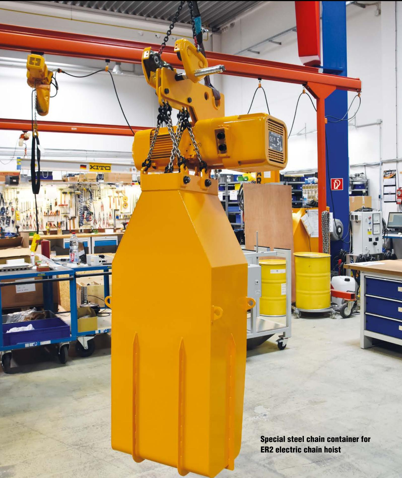
**Special steel chain container for ER2 electric chain hoist**
